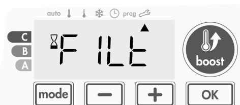
The blower continues to operate but does not heat up. Check if nothing is put in front of the ventilation grid to not block the air flow. The filter could be plug by dust, it must be cleaned (see page 19).
