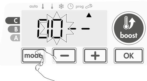
The PIN code is initialized, the next setting automatically appears: PIN Code activation.
