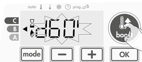
During the first minute, you can modify the Boost duration from 0 to the maximal authorised duration of the Boost, such as defined during the advanced settings (see page 12 for more details) by intervals of 5 minutes (or more quickly by push superior to 2 seconds) by pressing **-** and **+**.
