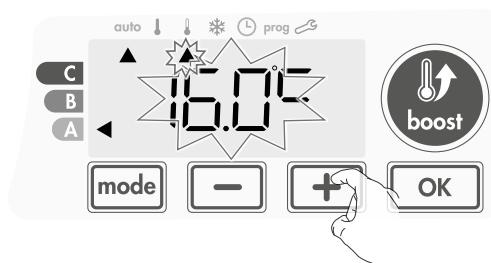
**Note:** The cursor corresponding to the operating mode, i.e Eco mode in our example, is blinking during the duration of the temporary derogation.
