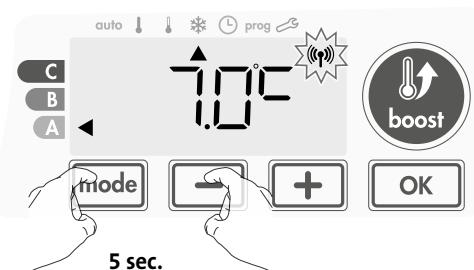
The **(RF)** symbol disappear from the display, the remote control and the blower are not associated.
